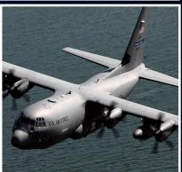
The C-130J Super Hercules represented a significant upgrade from the legacy C-130 aircraft like the C-130H. Equipped with six-blade Scimitar propellers, the C-130J had more powerful engines and an upgraded flight deck that included digital avionics.
